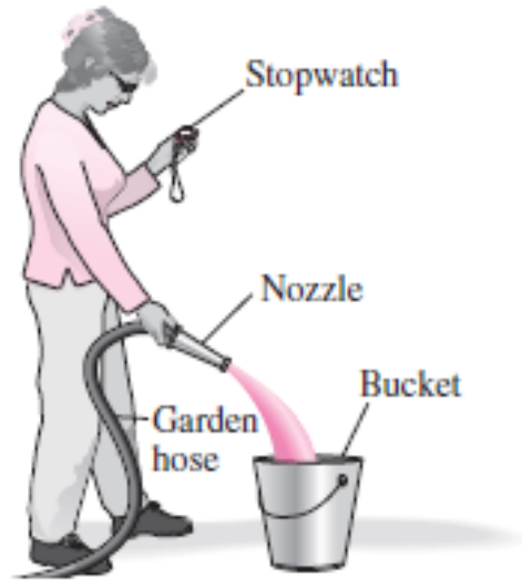
Fig 4.14: A primitive (but fairly accurate) way of measuring the flow rate of water through a garden hose involves collecting water in a bucket and recording the collection time.
