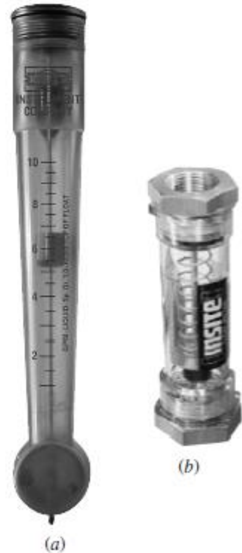
Fig 4.17: Two types of variable-area flow meters: (a) an ordinary gravity-based meter and (b) a spring-opposed meter.
